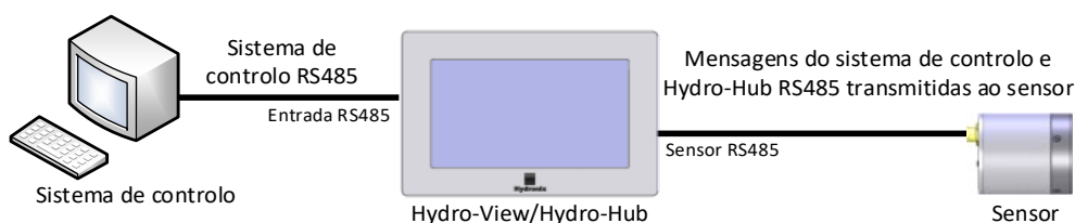
Figura 18: Hydro-View/Hydro-Hub a serializar a RS485
