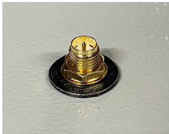
Figure 9: Antenna extension cable installed
