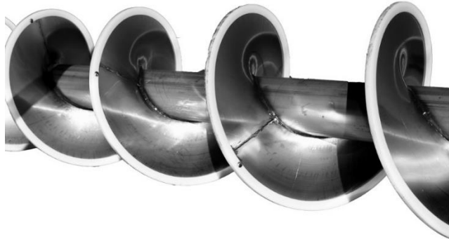
Figure 11: Flight Edging on a Screw Conveyor
