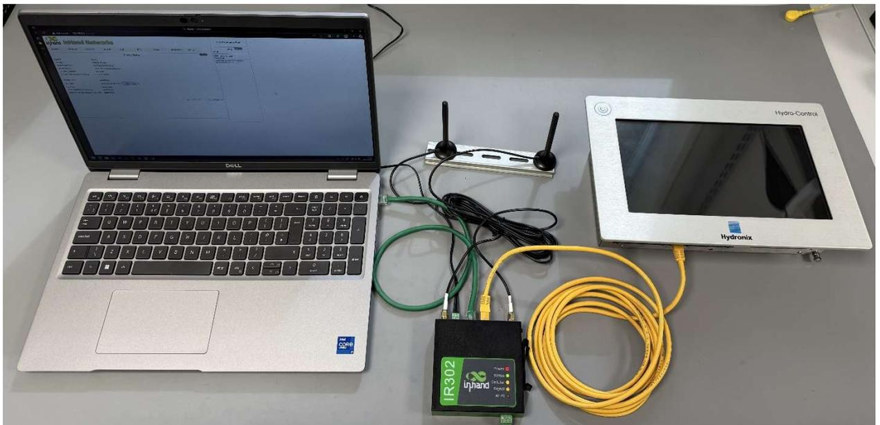
Fit the activated SIM card into Slot 1 of the SIM card holder and insert into the Router.
