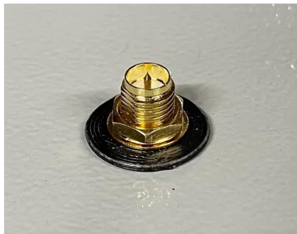
Figure 8: Antenna extension cable installed
