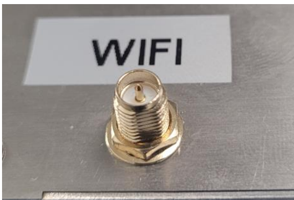
Figure 5: The Wi-Fi antenna connector
