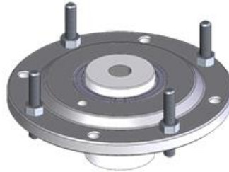
Figure 24: Mounting Studs installed
