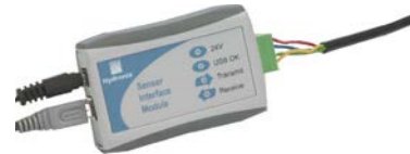
Figure 37: SIM01A USB to RS485 converter connections (SIM01A)
