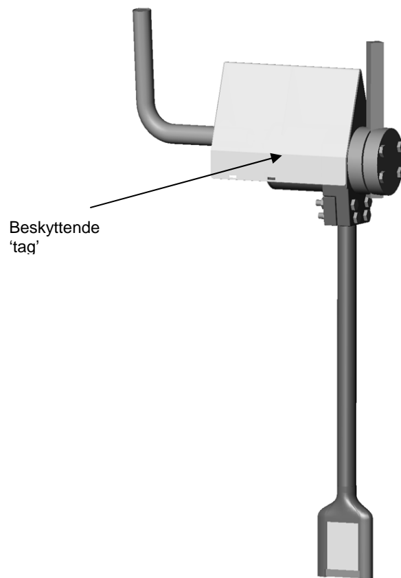
Figur 5 – Beskyttende 'tage' placeret over sensorlegemet
