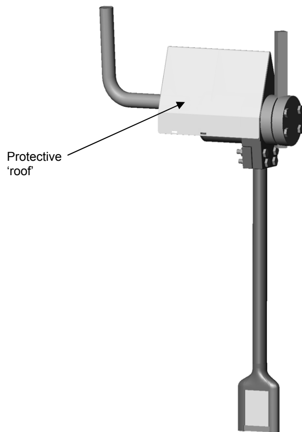
Figure 5 - Protective 'roof' placed over the sensor body
