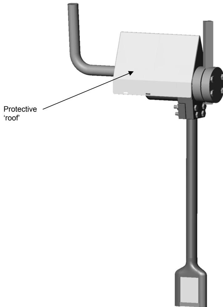
Figure 5 - Protective 'roof' placed over the sensor body
