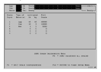
The same Scale inputs you have in your Probe Calibration Screen are the same 6 inputs used in the Scale configuration Screen. The Scale input used above cannot be used for Moisture Probes. By looking at the above example you will see that Scale Channels 1,2, and 3 are being used as Scales and are not available for use as Moisture Probe interface channels.
