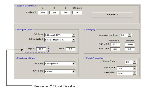
Note: The A, B, C, SSD values will change once the sensor is calibrated to the material.
