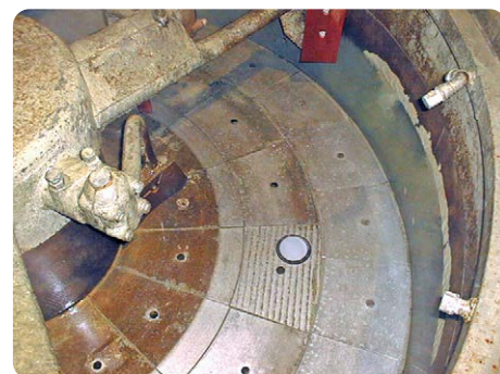
Sensor installed in a mixer
